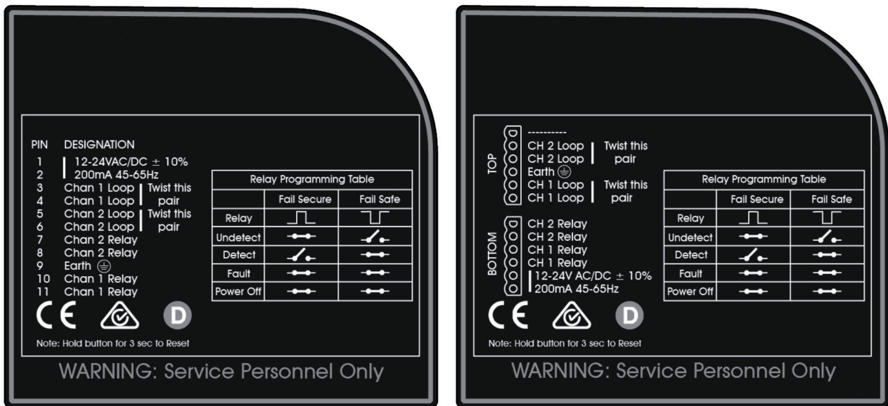
Figure 8. Example of LC20-2 Side Labels. Power supply requirements and pin connections are clearly stated on the side of the unit. 11 Pin configuration is shown on the left, DIN Rail on the right.
